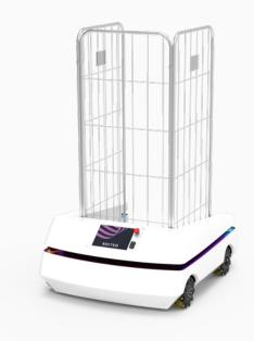
Solteq Trolley Robot moves autonomously carrying loads up to 400 kilograms. The robot can be integrated with other systems, such as elevators, used in the premises. Load-carrying solutions, such as platforms, are tailored to each customer's needs.
