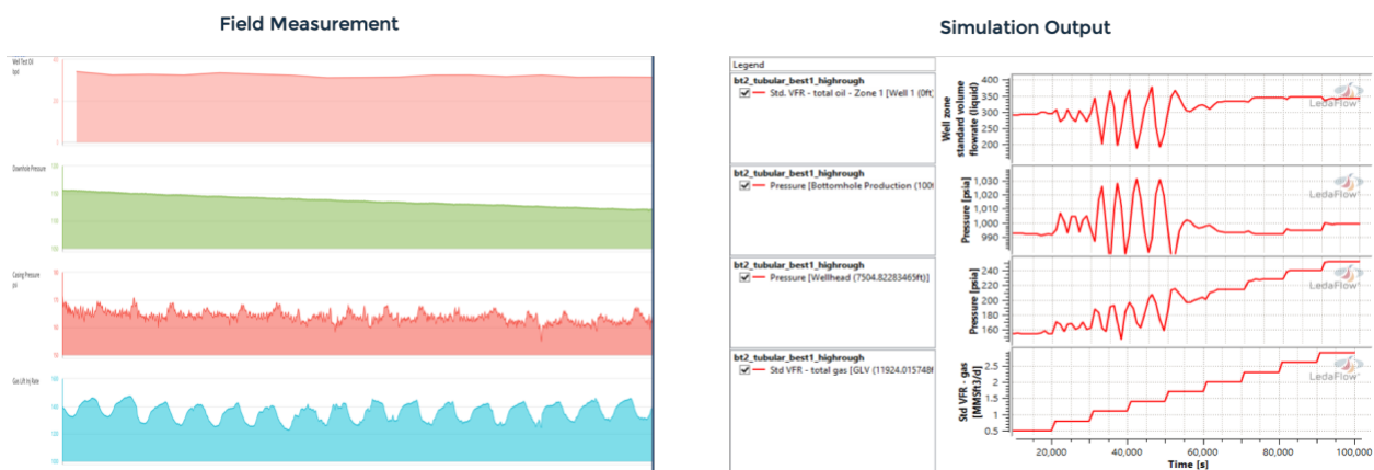
Fig. 11: Response comparison between field measurement and simulation output.
